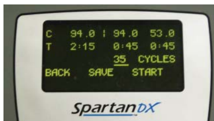
Figure 1. Screen appearance after the cycling parameters have been input in the instrument.
